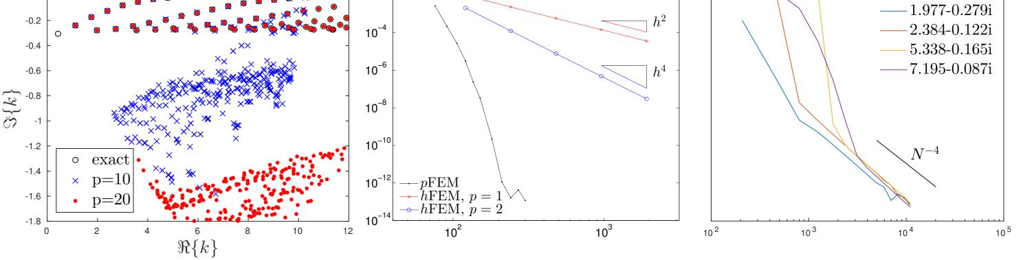
• In a) we show examples of spectral pollution from PML computations. It is evident that improving the mesh quality (increasing the polynomial degree **p**) moves spurious eigenvalues away from the area of interest.
